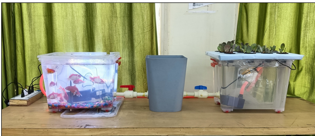
Fig. 3 : Experimental Aquaponics setup in integration with Deep water culture
